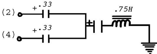
Schematic of passive audio tone filter
