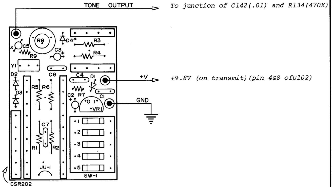
NOTE: Remove R133 (100K) on transmitter circuit board tone generator to disable internal tone generator.
