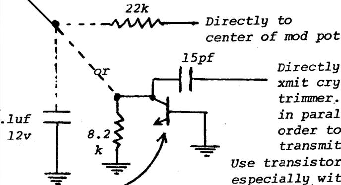
Any NPN silicon transistor with Emitter cut off.
