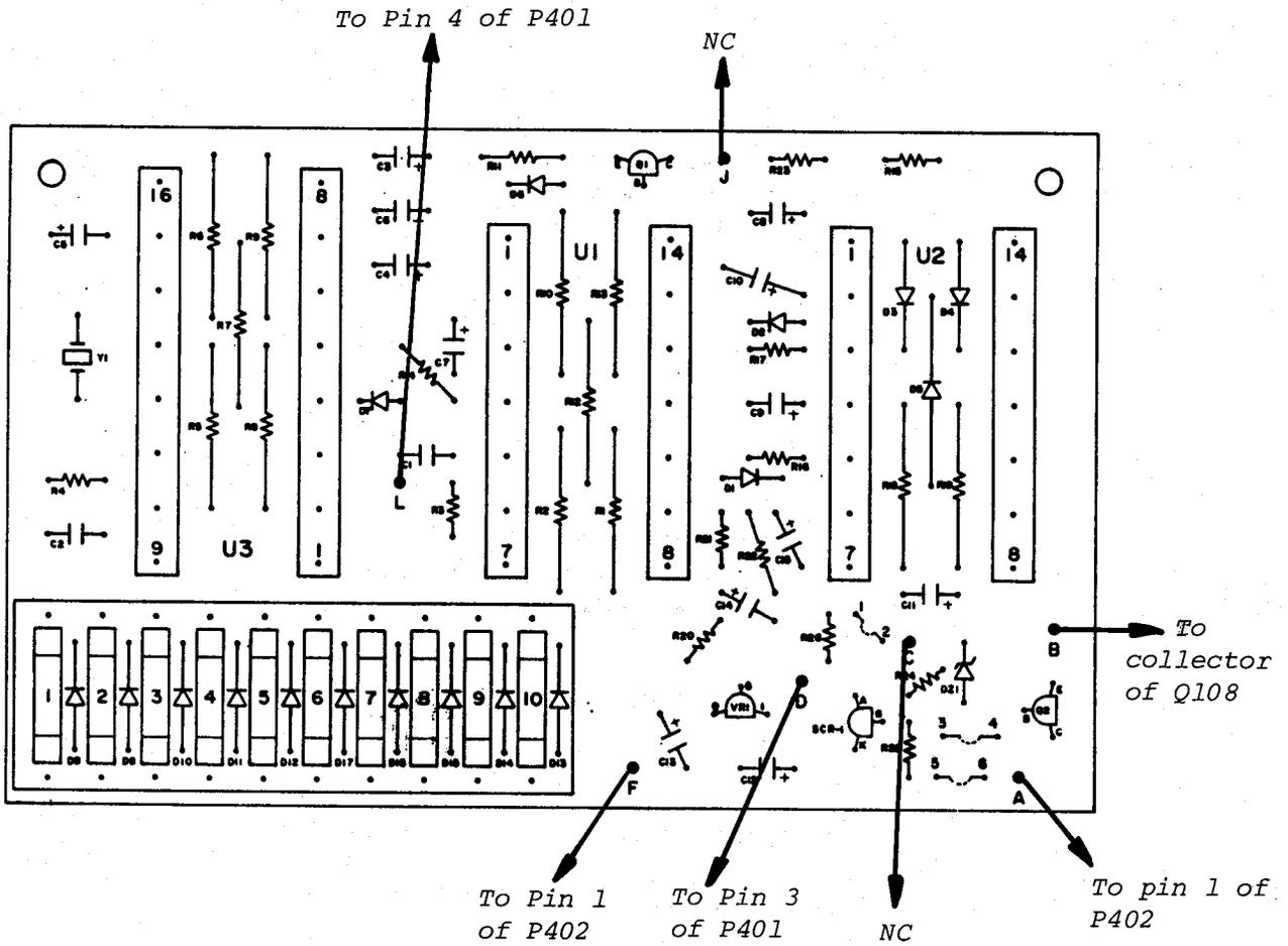
NOTE: Remove jumper from Pin 4 of P401 to pin 6 of P402 and replace with 100K resistor.
