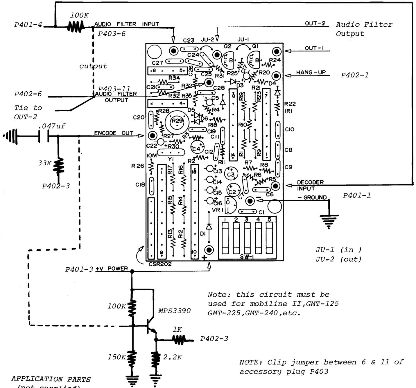
Note: this circuit must be used for mobiline II, GMT-125 GMT-225, GMT-240, etc.
