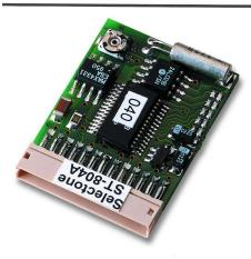
•All three popular signaling formats are available in one unit. PC Programmable encoder interfaces with all FM transceivers. Small size makes it perfect for handhelds and mobiles, and low profile connector makes programming and installation a snap. Uses ST-804PM Product Manager software, available for free from our web site, or at a nominal cost from our factory.
