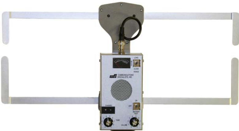
PR-100 SHOWN WITH FOLDING FA-3 ANTENNA.
