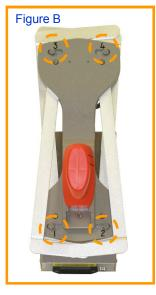
The directional antenna can be used in two ways. The PR-100A receiver can be mounted on the FA-3 antenna for one handed operation or the CA-4 coax assembly can be attached so that the antenna and receiver can be separated.
