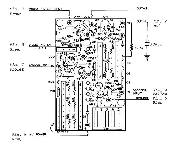
Notes: The Decoder is Modified by adding a 100uf cap. from Out. 1 to ground. A 3.9K resistor from Out. 1 to regulated 8vdc. on the decoder board.
