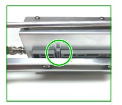
To detach the receiver from the antenna, push the release latch on the antenna mount and slide the receiver from the antenna. When re-attaching, slide the receiver forward until a small click is felt.
