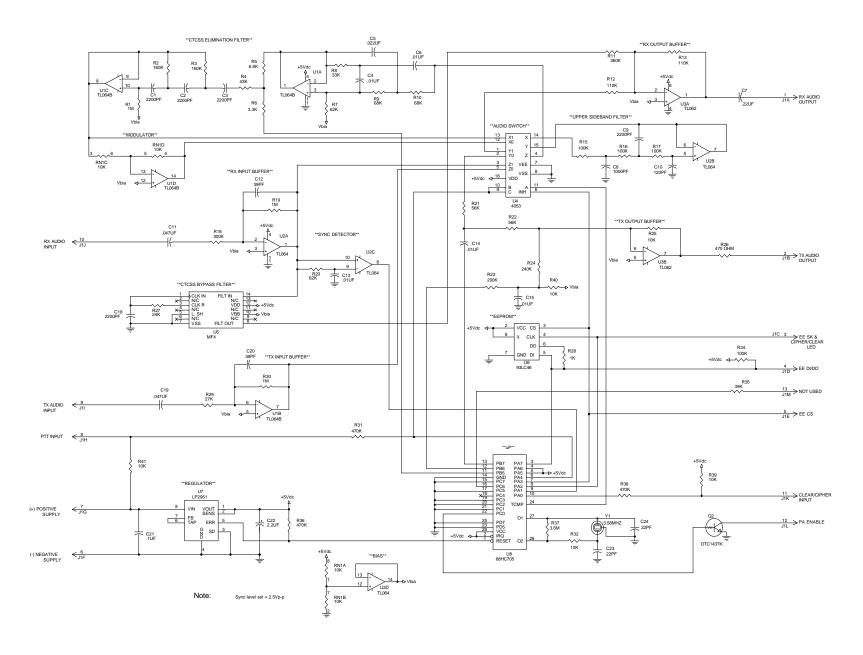
Figure 8 - ST-25AMC/AMT Schematic Diagram
