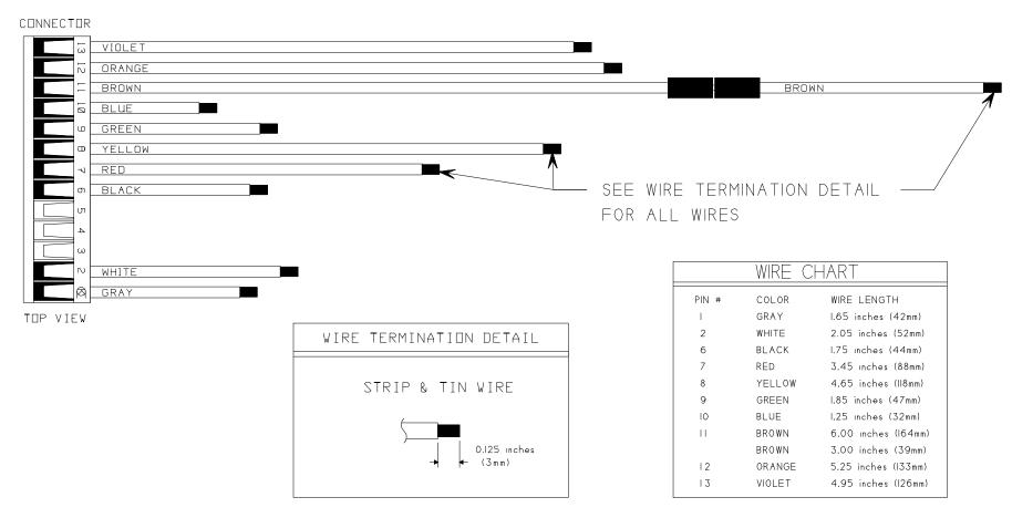
Figure 1 - ST-25AMC Cable Drawing
