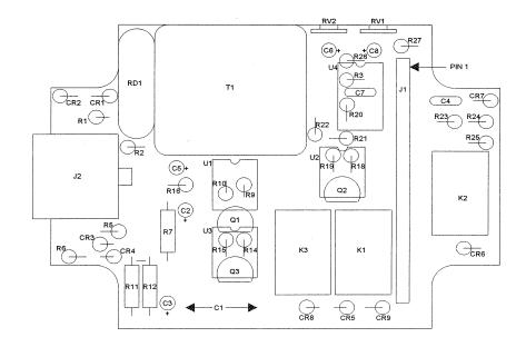
NOTES 1. THE TOP LEAD OF ALL DIODES IS THE CATHODE. 2. PIN 6 OF U1, U2 AND U3 MUST BE CUT OFF.
