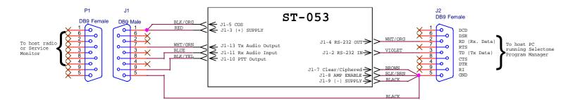
Common connections are soldered directly at the connector indicated on the schematic.
